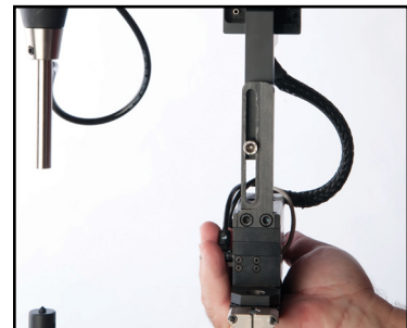
New T-bracket and shuttle with integrated connectors.
