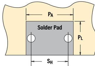
Solder pad can be flush to edge.
