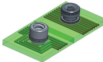
The SMTBSO™ fastener does not require a through hole allowing for copper traces to run under the fastener which better utilizes space on the board.
