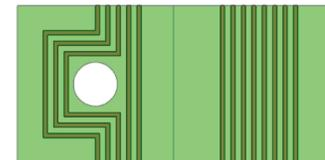
PC Board with through hole.    PC Board without through hole.
