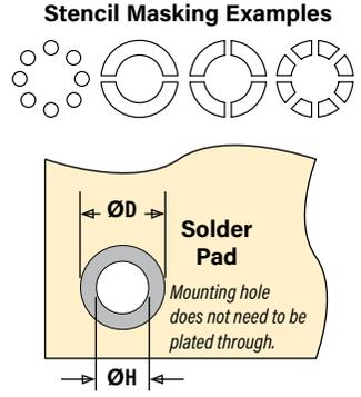
**NOTE:** Standoffs are available on special order without a pilot that do not require a thru hole for installation. Contact [techsupport@pemnet.com](mailto:techsupport@pemnet.com) for more information
