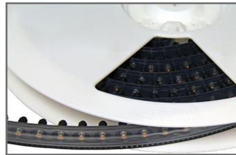
Packaged on 330 mm recyclable reels. Tape width is 24 mm. Supplied with polyimide patch for vacuum pick up. Reels conform to EIA-481.
