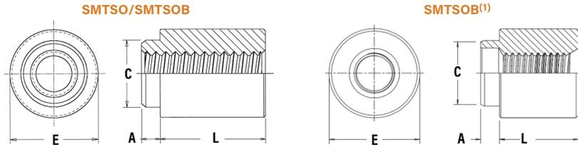
Thread/thru hole sizes 2-56, 4-40, 6-32, 8-32, 116, 143, M2, M2.5, M3, M3.5, M4, 3.1, 3.6, and 4.2
