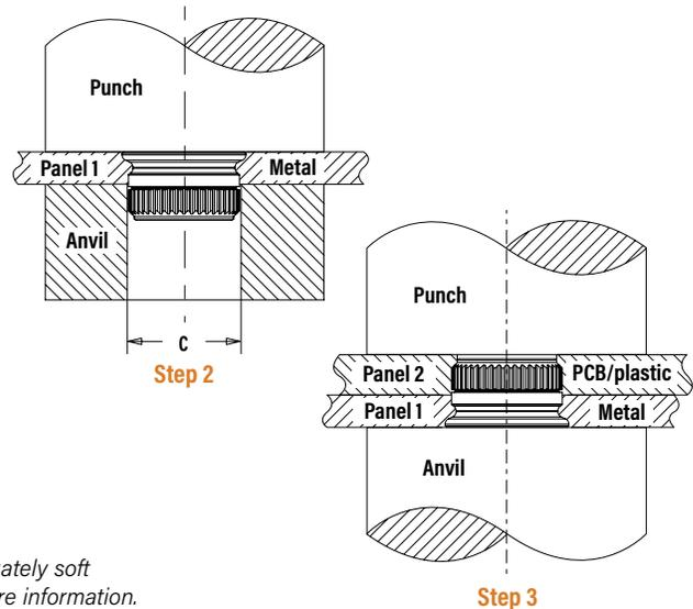
**NOTE:** Fastener can be installed in both sheets at once when metal panel is adequately soft compared to the non-metal panel. E-mail [techsupport@pemnet.com](mailto:techsupport@pemnet.com) for more information.
