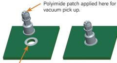
Solder paste applied to pad on PCB.
