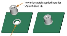
Solder paste applied to pad on PCB.
