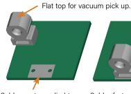
Solder paste applied to pad on PCB.
